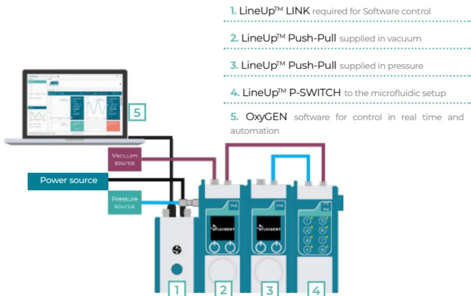
In this example, the Push-Pull [2] regulates pressure and vacuum, and provide vacuum to the P-SWITCH. The Push-Pull [3] regulates pressure and provides pressure to the P-SWITCH. Each independent outlet of the P-SWITCH can deliver pressure or vacuum to the microfluidic set-up
