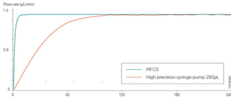
**FLUIGENT** Technology allows to obtain a fast flow rate response over the time . With a **short settling time** and **quick pressurization of systems**. Compared to syringe pumps, **MFCS™-EX** allows to save experimental time, precious samples and expensive reagents with significantly **shorter response times compared to syringe pumps**.
