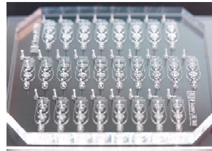
Fig. 2. Standard Drop-sequencing chip containing 26 individual Droplet Generation Devices.
