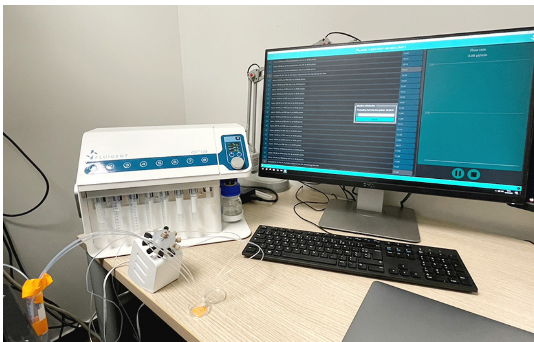
Figure 4: Photo of experimental setup showing Aria, M-switch, and Aria software.
