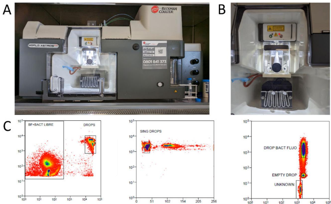
Figure 7: FACS machine used for sorting (A) with a zoom to the sorting area (B), and cytometry analysis and gating (C).
