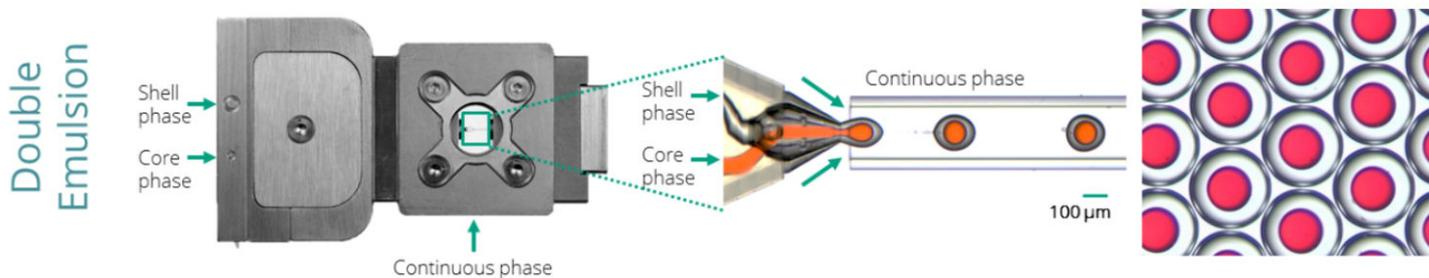
Figure 2: Structure of the Raydrop® [4].
