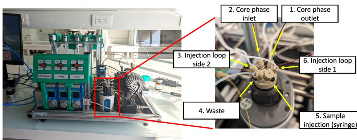
Figure 3: Double emulsion platform with injection loop.
