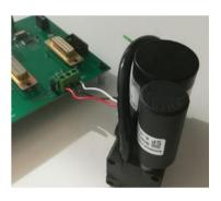
It is selected using the small jumper labelled "V ctrl" next to the terminal block. Its default state can be changed using the first switch of the 4way switch labelled "options". Note that the 5V is current limited
