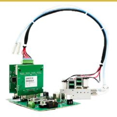
The F-OEM consists of a main platform – the integration board – that supports up to 8 modules: pressure modules (different ranges, push-pull), switch and electrovalve modules (for valve integration).
