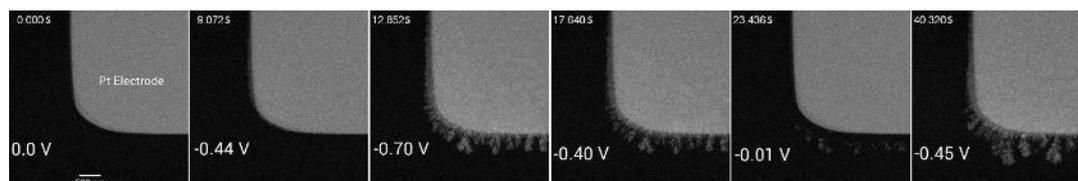
Figure 3. Time series of HAADF-STEM images illustrating the growth and etching process of Cu dendrites on the Pt electrode by employing cyclic voltammetry scanning. In the experiments, incident electron flux was set  $\sim 50 \text{ e nm}^{-2}\text{s}^{-1}$ , and the liquid flow rate was  $1.7 \mu\text{L}/\text{min}$ .
