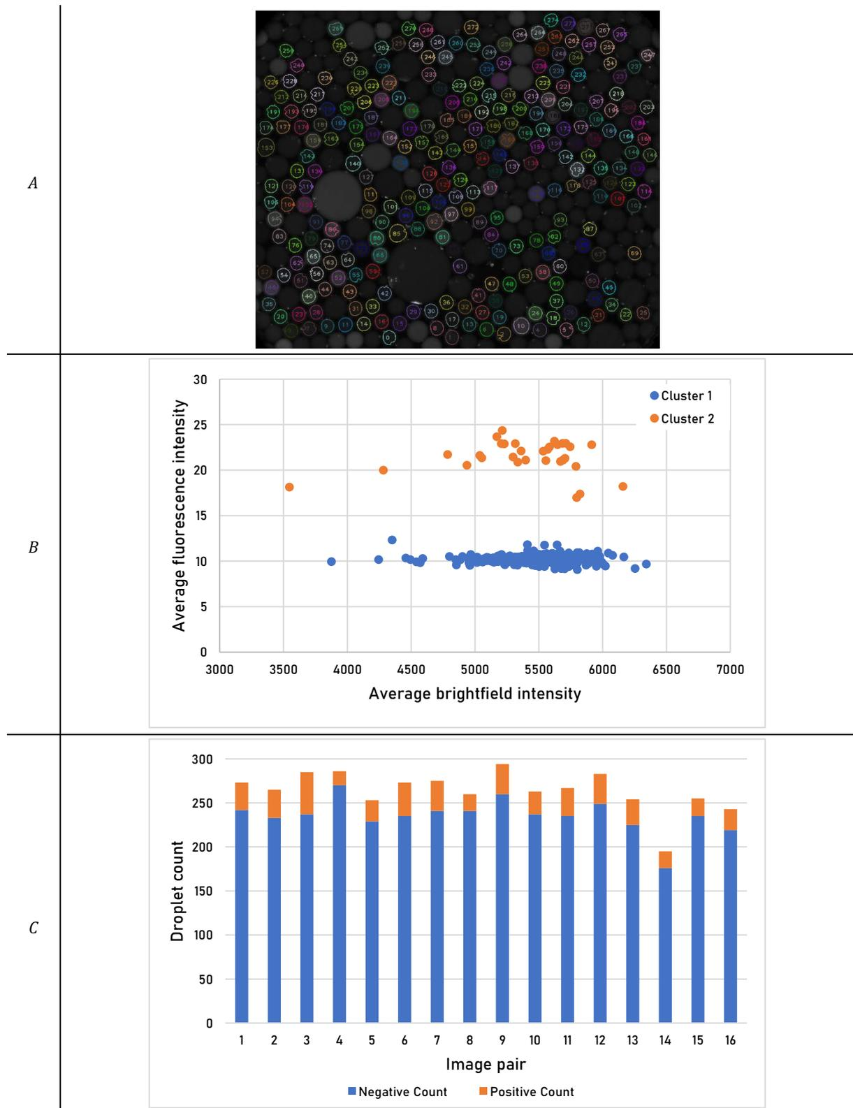
**Figure 5:** Digital PCR results compilation. A) Fluorescence readout image example with spots, used for droplet measurements. B) Clustering scatter plot, showing the separation of the positive and negative droplets based on their
