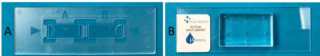
**Figure 1:** Utilized chip devices: A) 10 µl cell counting chamber B) Fluigent PDMS EZ Drop chip
