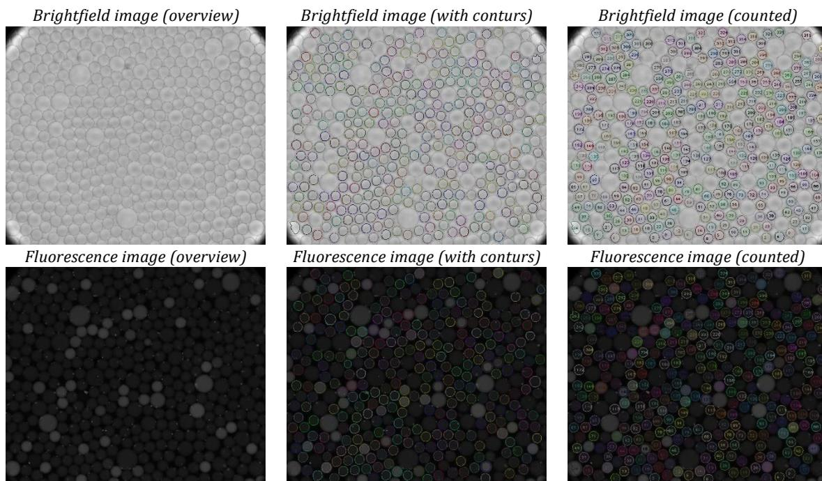
**Figure 4:** Evaluation procedure for the dPCR. Starting point are brightfield and fluorescence images of the generated droplets. The processing is done by a self-developed software to detect and evaluate the intensity of the droplets. The parameters for detecting the droplet contours are defined in advance. Only droplets of a valid size are included in the result.
