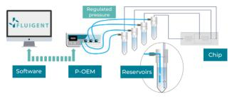
The original pneumatic path combined with a very fast regulation algorithm has been developed to deliver regulated pressure from a pressure source. The principle of pressure actuation in microfluidic systems is shown in the figure above and the benefits of this technology are listed below.
