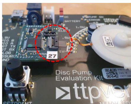
Figure 3: FPC connector in closed and open positions
