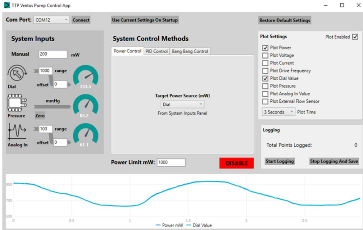
Figure 6: power controlled to a target controlled by the SETPOINT dial on the motherboard.
