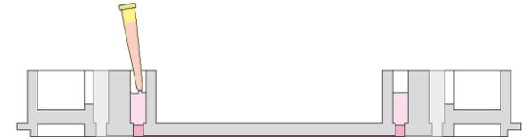
**6. Add medium to the reservoirs** to fill the lateral channels. **Cover and incubate** until needed.
