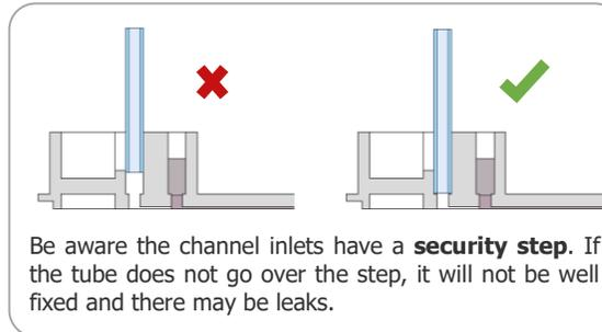
Be aware the channel inlets have a **security step**. If the tube does not go over the step, it will not be well fixed and there may be leaks.
