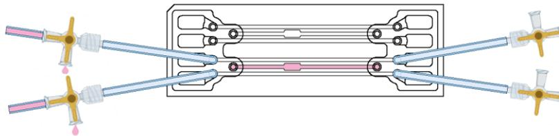
6. When medium has filled the tube from the perpendicular entrance in both inlet stopcocks, **stop the flow, open the inlet and outlet stopcocks** and reactivate the flow to let the medium pass through the lateral channels.
