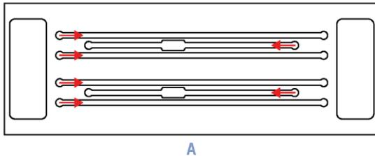
The central **culture chamber** must be **completely dry** in order to confine the hydrogel in it.
