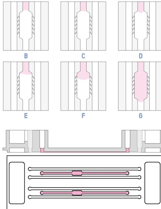
**4. Flip the chip upwards and downwards** every 10 seconds for a few minutes for **homogeneous 3D distribution** during the polymerization of the hydrogel. Incubate at manufacturer's conditions.
