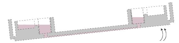
**Note:** Another way to proceed is to **pipette the solution into the inlet well** and let the liquid to flow by itself through the channel until it reaches the outlet well.
