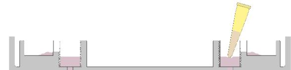
**Important:** Note that the channel should never dry up. Take incubation times into account and use the evaporation reservoirs as long as possible.
