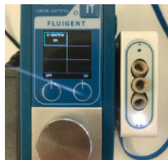
2-SWITCH™ in position 2
