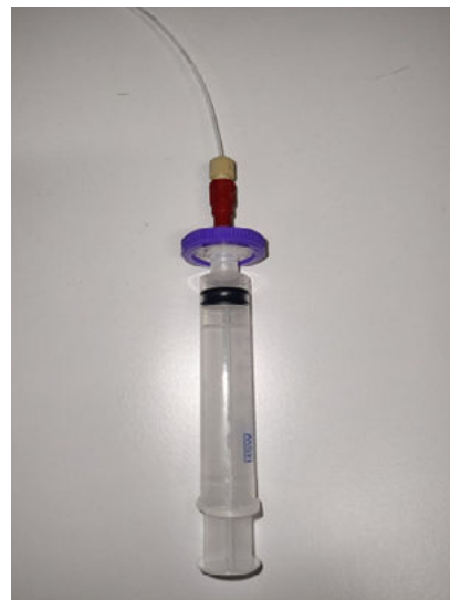
Figure 26: Purge the continuous phase
