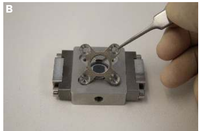
Figure 26: Dismantling the RayDrop A) Removing the screws B) Removing the X-shaped metallic
