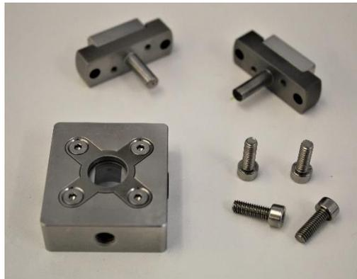
The RayDrop is a versatile device. Components including the Nozzle and collecting capillary are easily exchangeable. This allows one to target different droplet sizes as well as for potential cleaning if needed.
