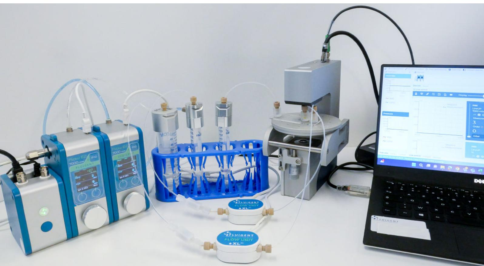
**The Fluigent Liposome Production Package is a versatile, high-quality system to control the production of monodisperse liposome nanoparticles. It allows the user the flexibility to vary the size of the nanoparticles produced. The high performance of the system comes from the combination of Fluigent's LineUP microfluidic pumps and the Little Things Factory (GmbH)'s staggered herringbone mixer, a reusable glass microfluidic chip.**
