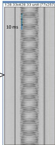
The stack of pictures was then compiled, in Z line projection. Black strip = droplets / White strip = no droplets/
