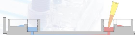
**Tip:** You may **tilt the device** manually in order to make the dilution buffer flow **several times** from one reservoir to another before removing it.
