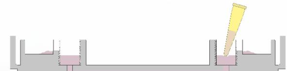
**Important:** Note that the channel should never dry up. Take incubation times into account and use the evaporation reservoirs as long as possible.
