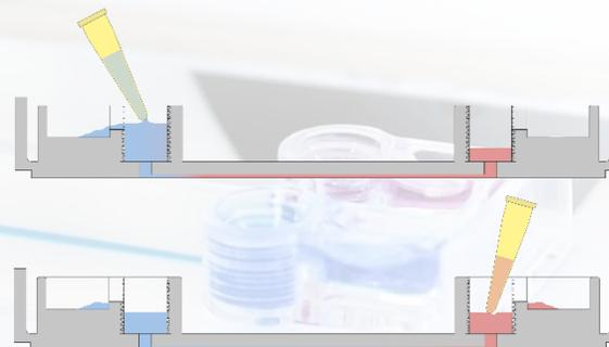
**Tip:** You may **tilt the device** manually in order to make the dilution buffer flow **several times** from one reservoir to another before you remove it.
